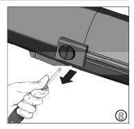
**Note:** The brush must be inserted with its black part directed inside the motor.
